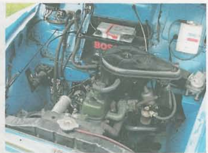
Engine bay was designed to take a flat-four, and the Minor had an extra four-inch width added at the last minute. All of which means there's lots of room round the bay for routine servicing – and, if it appeals, fitting a twin-cam Fiat engine or similar.
