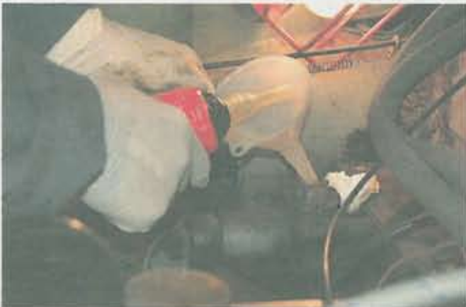
This is typical of the sort of thing you can do with Minors. You don't have to renew shock absorbers; provided the leak isn't too bad you can usually restore action by simply topping up – use hydraulic jack oil if you can't get shock absorber fluid.
