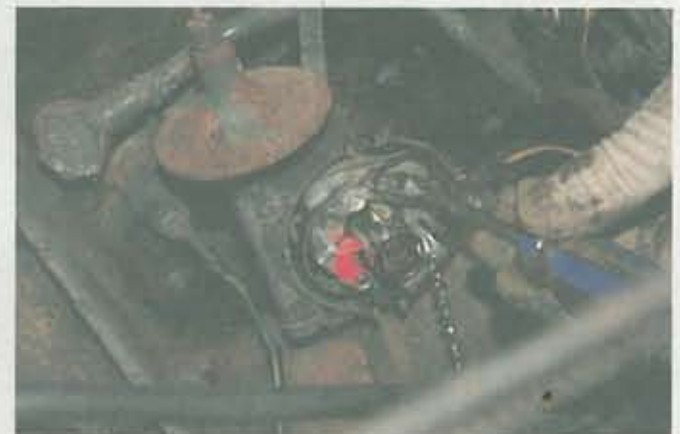
Distributor servicing is also straightforward due to excellent access. As always, it's sensible to renew the condenser and rotor arm at the same time as you change the points. There's even a starting handle to help you get the centre spindle positioned correctly.
