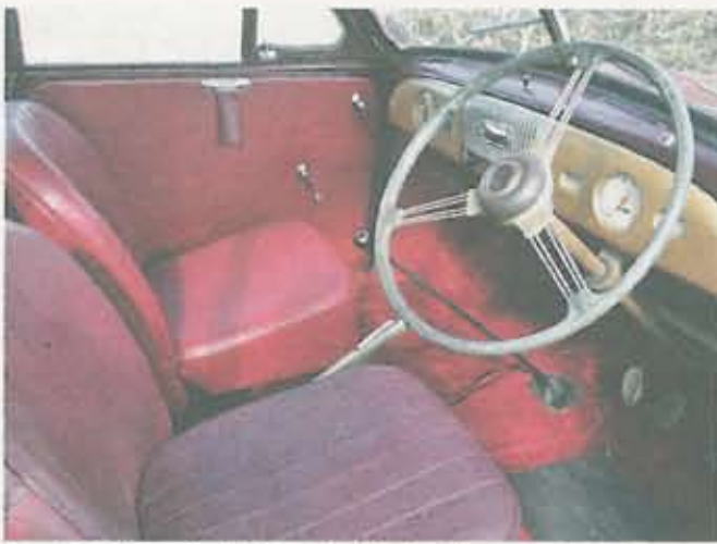
Pre-1954 Minors had this style of dash with a speedometer in front of the driver rather than centrally mounted. Note the matching decoration on the nearside, allowing the same basic dash shell to be used for LHD and RHD versions.
