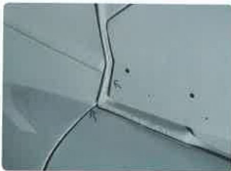
12 Elsewhere, getting the rest of the bodywork to fit nicely has meant a few compromises. The Charles Ware team weren't happy with the fit of our driver's door, and that meant dressing the A-pillar area forwards slightly. The door and wing now cooperate nicely but again the paintwork needs touching in – another reason not to send a car for paint until every last panel has been checked for fit.
