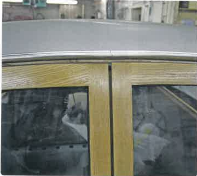
7 The mouldings are fitted as two separate pieces, with the join above the rear doors. Attention to detail here sees the join end up dead in the centre and neatly aligned.
