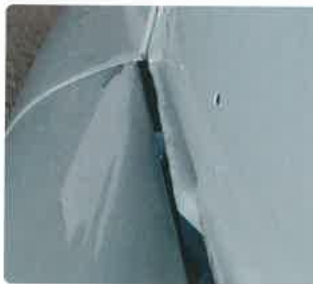
13 This is the combination of the extensive welding work the car has received and the use of a pattern wing. To get the wing to sit flush with the door skin, the fitting bolts have been packed out. It's not unusual with wings that don't fit brilliantly.
